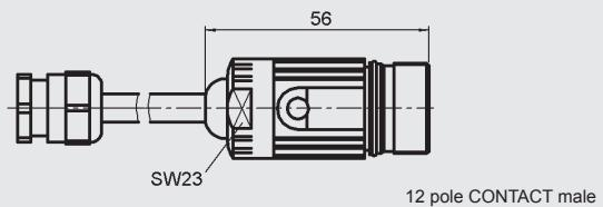
Signal output: Synchronous Serial Interface (S01):
